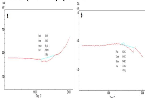
**Fig. 9:** DSC curves of (a) composite with 9 wt% Ag NPs (b) ABS
