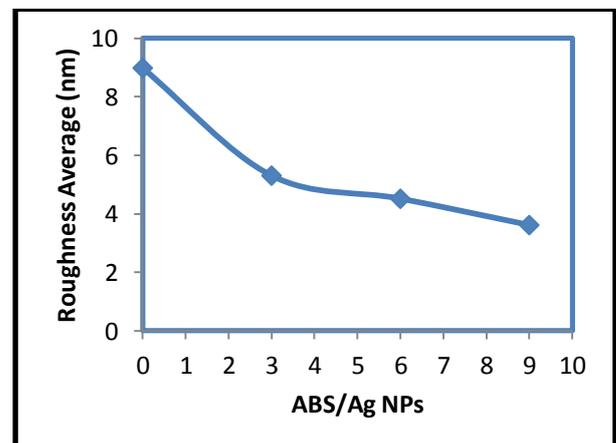
Fig. 8: Roughness average as a function of Ag NPs content
