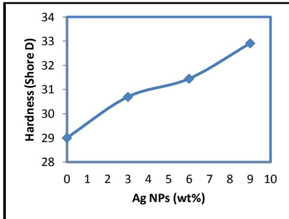
Fig. 4: Hardness as a function of Ag NPs content
