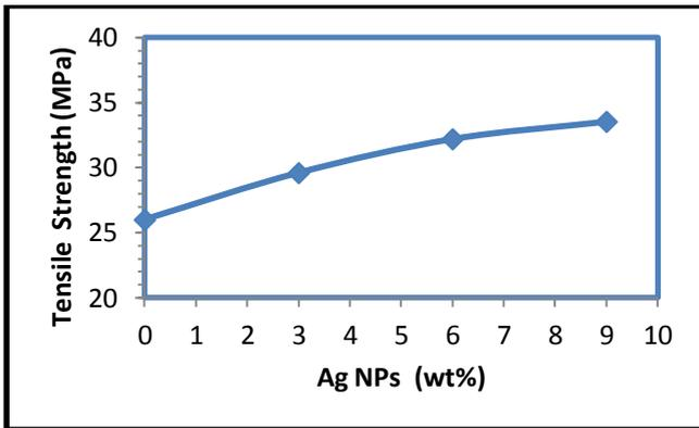
Fig. 3: Tensile strength as a function of Ag NPs content
