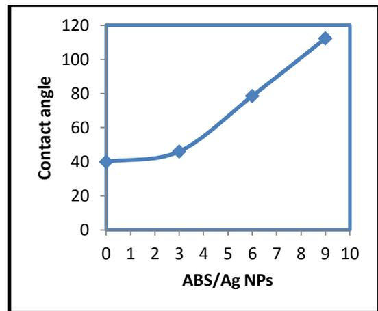
Fig. 7: Contact angle as a function of Ag NPs content
