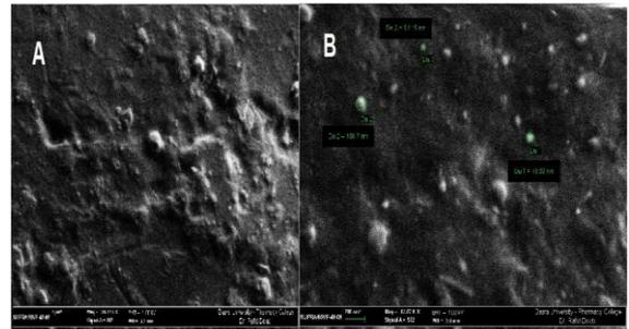
**Fig. 10:** SEM image of (a) ABS (B) composite with 9 wt% Ag NPs
