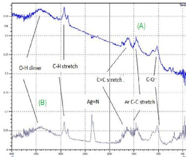
Fig. 5: FTIR spectra for (a) pure ABS (b) composite with 9 wt% Ag NPs
