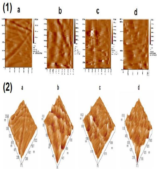
**Fig. 9:** Surface nature as a function of Ag NPs content (1) 2D images (2) 3D images (a) Pure (b) 3 wt% (c) 6 wt% (d) 9 wt%
