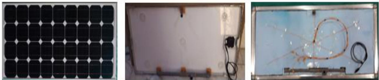
a:PV module b:Channel of Cooling Water c:Back Side of PV/T System Fig. 1: PV Module and Parts of PV/T Solar System
