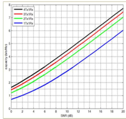
Fig. 6: Channel capacity of MISO
