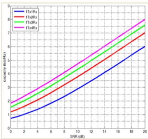
Fig. 5: Channel capacity of SIMO
