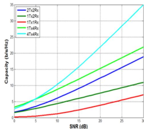
Fig. 8: MIMO and SIMO Channel Capacity Comparison
