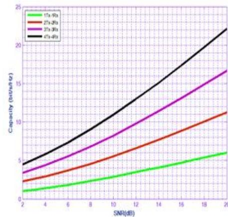
Fig. 7: MIMO system capacity with CSI at transmitter
