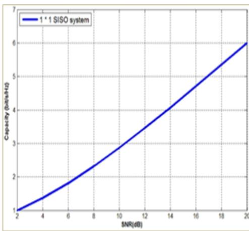
Fig. 4: Channel capacity of SISO
