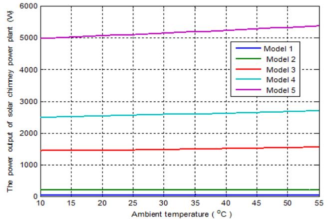
Fig. 6: The power output of solar chimney power plant with ambient temperature
