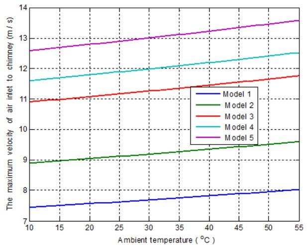
Fig. 7: The maximum velocity of air inside the chimney with ambient temperature
