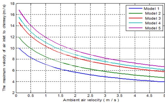
Fig. 3: The maximum velocity of air inside the chimney with ambient air velocity
