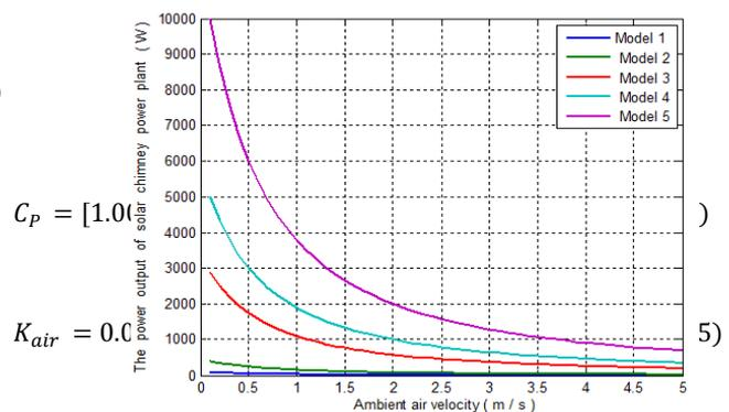
Fig. 2: The output power of solar chimney with ambient air velocity
