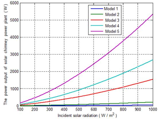
Fig. 5: The power output of solar chimney power plant with incident solar radiation
