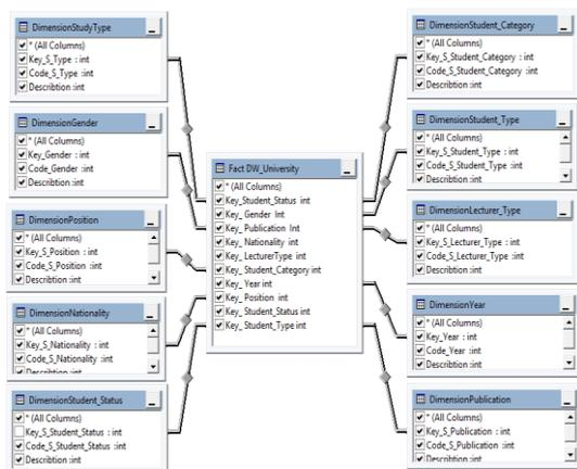
Fig. 5: DW Dimension Model (Star Schema)
