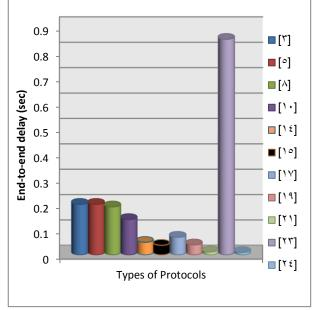
Fig. 1: Comparison of End-to-End Delay (Node Speed=10m/S).
