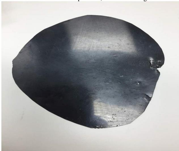
Fig. 1: Samples of graphene-epoxy TIM is formed
