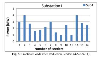
We can see from the Fig.5 that all feeders will be kept in operation and that means there is no shedding of loads but reduction only the feeder (4-5-8-9-11). In addition, from the Fig.4 the feeders (4-5-9-11) at first substation are switching off and their values will be 0 MW. But in Fig.5, the feeders (4-5-8-9-11) are being reduced their values from 12.8 MW to 6.62MW. To explain the variance of the LS scheme with and without  $\beta_{nm}$ , Fig.6.
