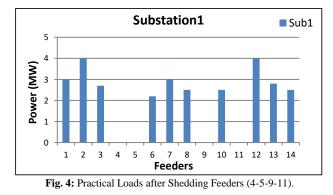
We can see that the feeders (4-5-9-11) are switching off (i.e. their values 0 MW) because they have a low importance factor. The aforementioned 4 feeders will be under shedding from the substation 1 in order to investigate the balance between the demands - supply power.
