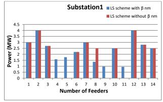
Fig. 6: Practical Loads after Reduction Feeders (4-5-8-9-11).
