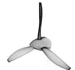
Fig. 2: Computational mesh (coarse mesh is shown)
