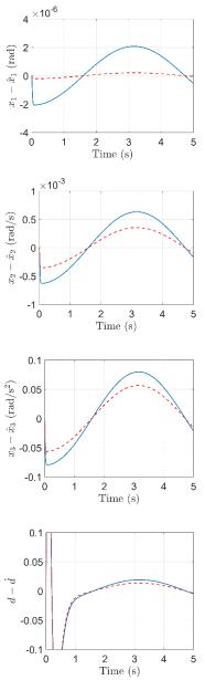
**Fig. 6:** Case-IV: Comparative Performance of Linear ESO (Solid Line) and Nonlinear ESO (Dashed Line) in the State and Disturbance Estimation Errors: (A)  $x_1 - \hat{x}_1$ , (B)  $x_2 - \hat{x}_2$ , (C)  $x_3 - \hat{x}_3$ , (D)  $d - \hat{d}$ .
