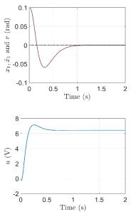
**Fig. 4:** Case-II: Motor Position and Its' Estimation and Control Input with Constant Load Disturbance: (A)  $x_1$  (Solid Line),  $\hat{x}_1$  (Dashed Line) and *r* (Dotted Line), (B) r.
