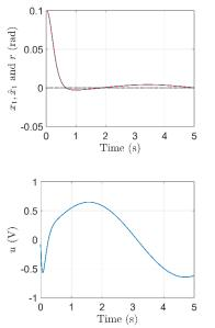
**Fig. 5:** Case-III: Motor Position and Its' Estimation and Control Input with Sinusoidal Load Disturbance: (A)  $x_1$  (Solid Line),  $\hat{x}_1$  (Dashed Line) and *r* (Dotted Line), (B) u.
