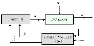
Fig. 1: The Block Diagram of the Overall Scheme.
