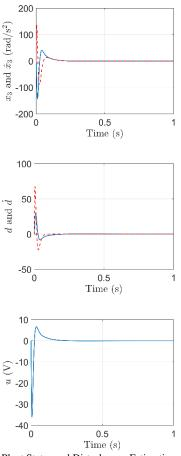
**Fig. 2:** Case-I: Plant States and Disturbance, Estimation and Control Input: (A)  $x_1$  (Solid Line),  $\hat{x}_1$  (Dashed Line) and r (Dotted Line), (B)  $x_2$  (Solid Line) and  $\hat{x}_2$  (Dashed Line), (C)  $x_3$  (Solid Line) and  $\hat{x}_3$  (Dashed Line), (D) d (Solid Line) and  $\hat{d}$  (Dashed Line), (E) u.
