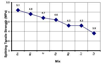
Fig. 3: Results of Splitting Tensile Strength
