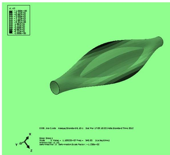
Figure 12: The displacement in the z-direction
