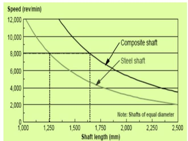
**Figure 1:** the relationship between shaft's length and the critical speed for both types of drive shafts
