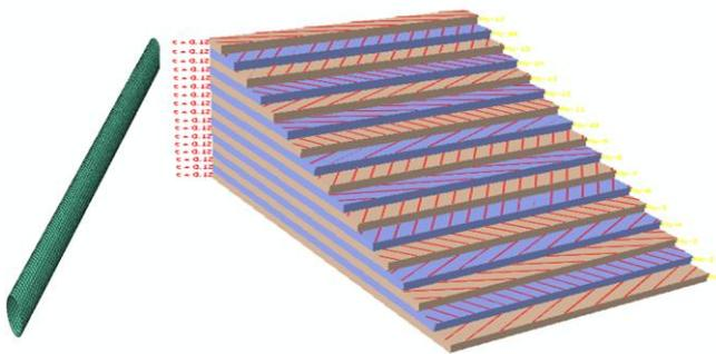
Figure 6: Visualization of ply stack
