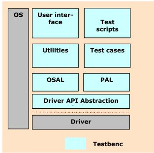
Fig. 4:Test-Bench Architecture.
