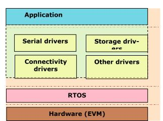
Fig. 2:Software Stack with Device Driver Layer.
