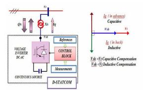
Figure: Basic model of DSTATCOM connected to the network
