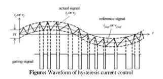
The real current is constrained to track the sine reference inside the hysteresis band by forward and in reverse (or impact) trading of the upper and lower switches. The inverter by then essentially transforms into a present source with crest to top current swell, which is controlled inside the hysteresis band, which makes the source current to be sinusoidal.
