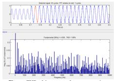
Figure: THD of the source after compensation.
