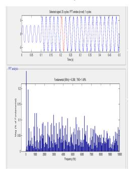
Figure: THD of the source after compensation with fuzzy logic controller.
