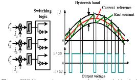
Figure: PWM hysteresis current control and its switching logic
