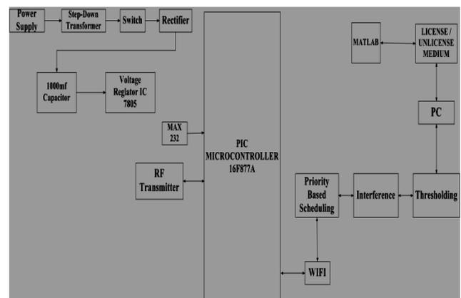
Figure 3: Block diagram for Transmitter side
