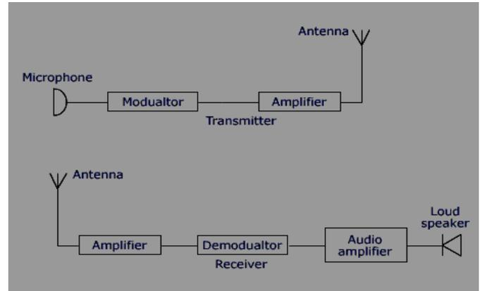
Figure 6: RF Transmitter /Receiver Diagram
