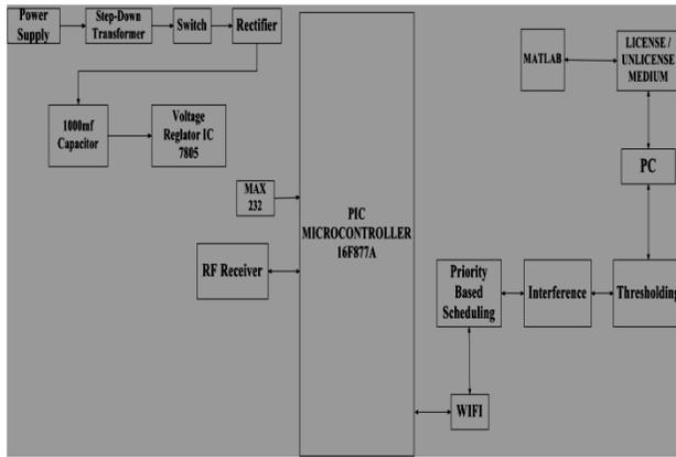
Figure 4: Block diagram for Receiver side
