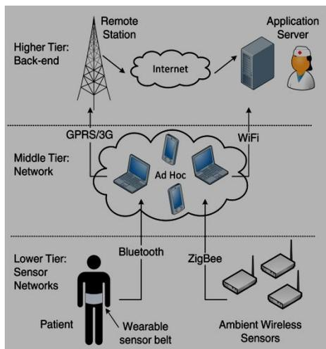
Figure 1: Three tier network architecture
