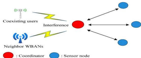
Figure 2: Conceptual operation in cognitive-receiver initiated cycled receiver (C-RICER).
