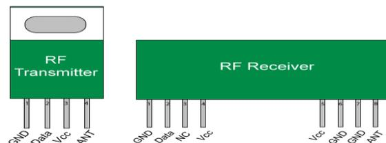
Figure 7: RF Transmitter /Receiver Pin Diagram
