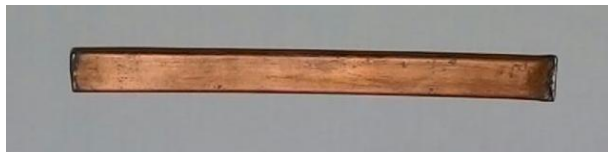
Fig. 4: Copper-Water s flat s heat s pipe
