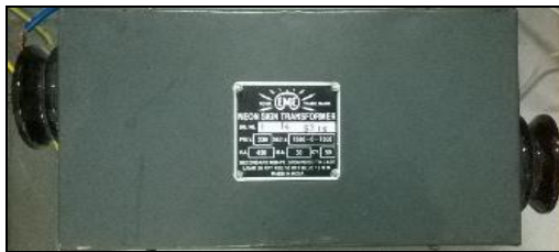
Fig. 3: Neon sign transformer
