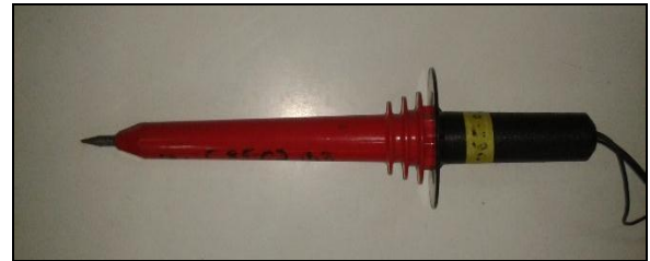
Fig. 5: High Voltage Probe
