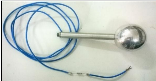
Fig. 9: Spark gap with resistor to limit current in the circuit
