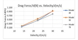
Fig. 13. Variation of F<sub>D</sub> with velocity (Experimental)
