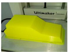
Fig 4: Printed car model
