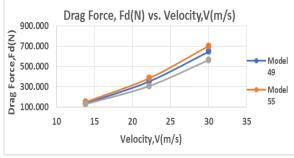
Fig. 14. Variation of  $F_D$  with velocity (Simulation)
