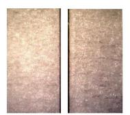
Fig. 8: Shear Edge Cohesive Failure Under A Stereozoom Microscope (Shear Zone) with A 75x Magnification.
