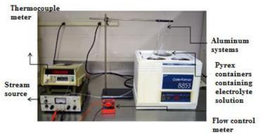
Fig. 3: PAA Setting with Voltage and Temperature Measuring Devices for Constant Monitoring.
