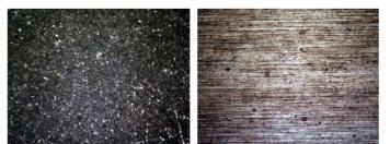
Fig. 1: Surface of the Sandblasted Aluminium T3-2024 (Left) in Comparison with A Similar Surface with Abrasion (Right) with 40x Magnification.
