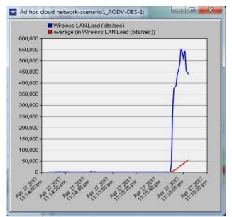
Fig. 14: Load (bits/sec) of Wireless LAN and average Load (bits/sec) of Wireless LAN of AODV
