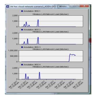
Fig.12: Network Load (bits/sec) of Wireless LAN of AODV for BSS1, BSS2, BSS3, and BSS4
