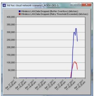
Fig 15: Data Dropped (Buffer Overflow) (bits/sec) and Data Dropped (Retry Threshold Exceeded) (bits/sec) of Wireless LAN and average Load (bits/sec) of Wireless LAN of AODV
