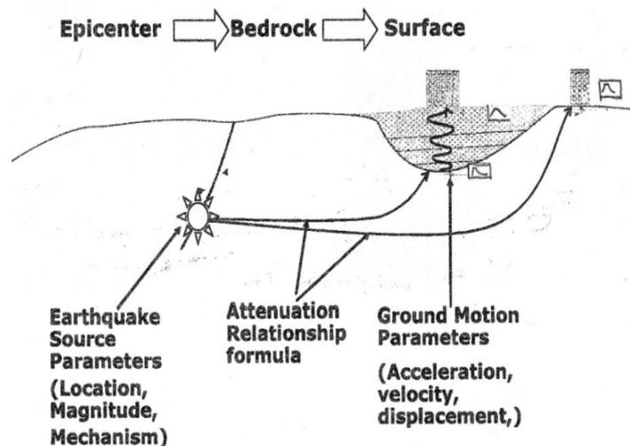
Figure 1: The illustration of wave propagation through soil surface and engineering bedrock [4].
