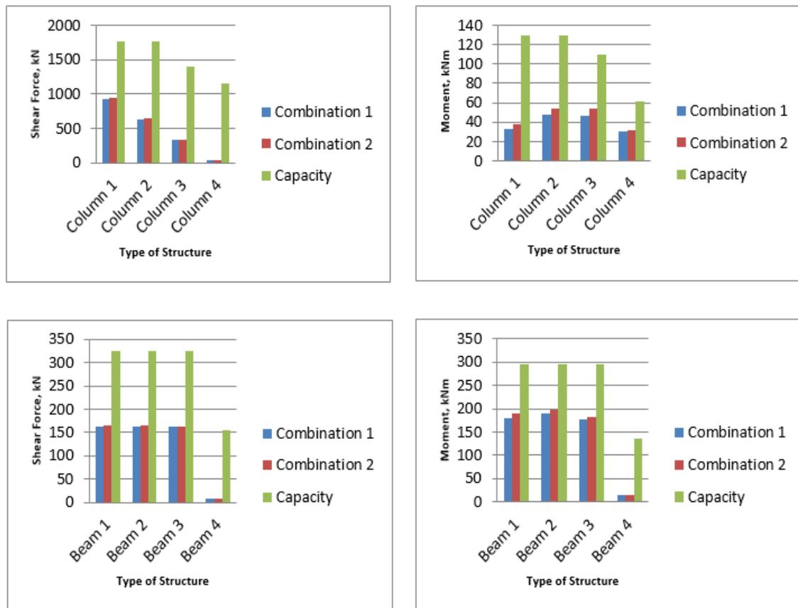
Figure 5: Analysis on Shear Force and Moment at columns and beams for Kuala Lumpur based fault zone.
