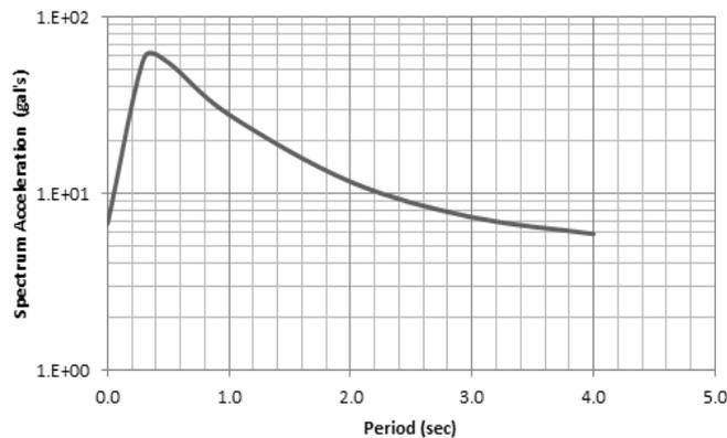
**Figure 3:** The spectrum acceleration analysis for fault zone in Pulau Pinang
