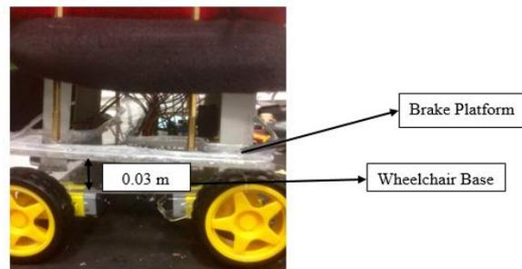
**Fig. 6:** The brake platform
