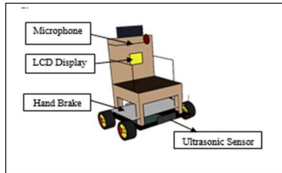
Fig. 2: The front-side view, of the wheelchair prototype
