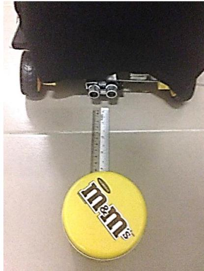
Fig. 12: Placement of the object from the ultrasonic sensor
