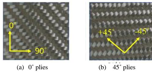
Fig. 6: Direction of fiber plies
