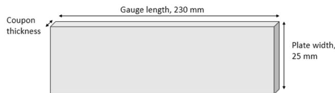
Fig. 1: Unnotched plate geometry
