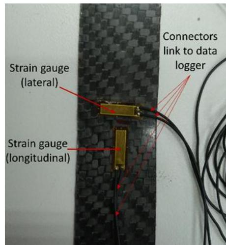
**Fig. 2:** Strain gauges was placed in both longitudinal and lateral direction connected to data logger
