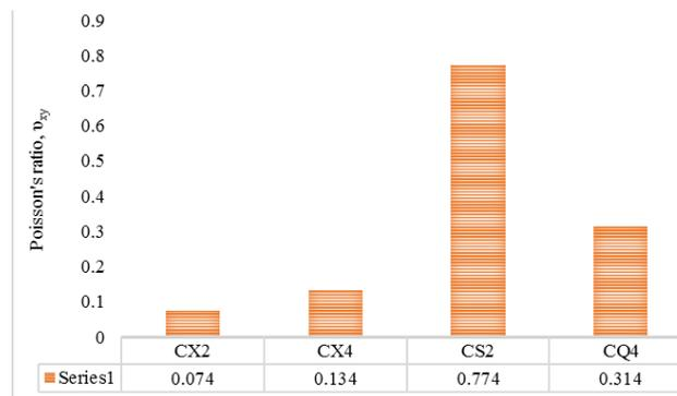
Fig. 8: Poisson's ratio for CFRP lay-ups
