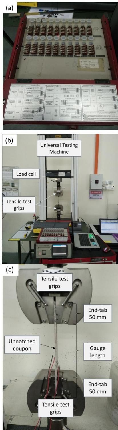
**Fig. 4:** (a) Data logger for strain gauge reading (b) UTM Machine tensile test set up connecting to data logger (c) unnotched coupon set up with strain gauges
