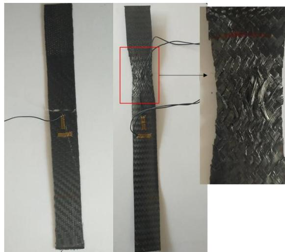
(a) Failure within gauge length (b) Fiber twisted within the coupon
