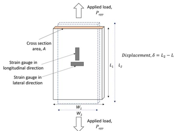
**Fig. 3:** Strain measurement as load applied by using strain gauge
