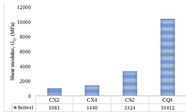
Fig. 9: Shear modulus for CFRP
