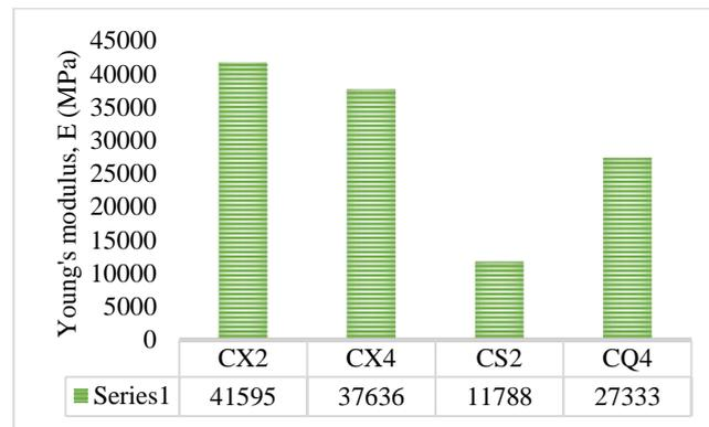
Fig. 7: Young's modulus for CFRP lay-ups
