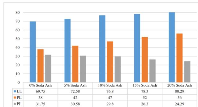
**Fig. 1:** The effect of the various soda ash percentages on the laterite soil's Atterberg limits. LL = Liquid Limit, PL = Plastic Limit, PI = Plasticity Index.
