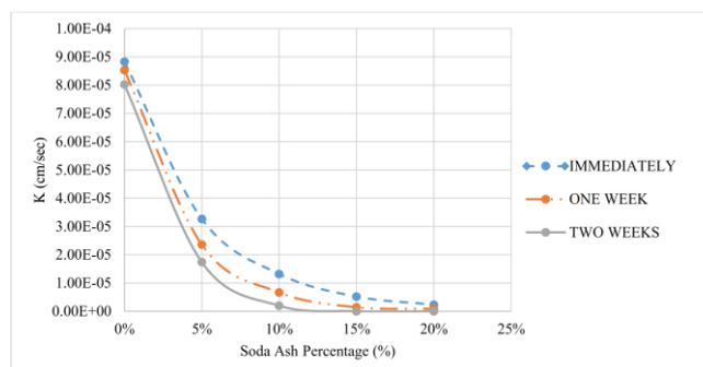
**Fig. 3:** Decreasing permeability coefficient according to the different sodium carbonate percentages and curing times
