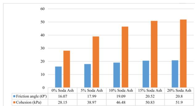
**Fig. 2:** The effect of various soda ash percentages on the laterite soil's shear strength characteristics
