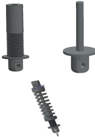
**Fig. 6:** Parts of mono-shock helical suspension spring
