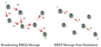
Fig.2: Ad Hoc On Demand Distance Vector Routing Protocol
