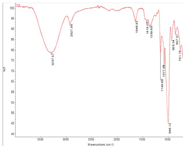
**Fig. 1:** FTIR Spectrum of starch in Potato Peel Waste
