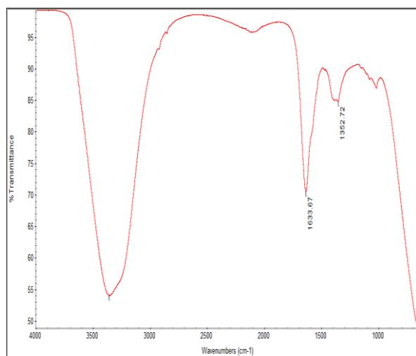
Fig.3: The FTIR spectrum of Gluconic acid
