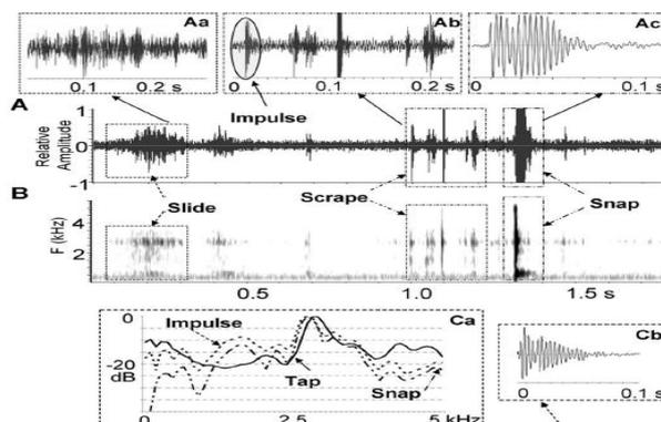
Fig. 4 Spectral and temporal pattern for insect infestation due to activity of insect.
