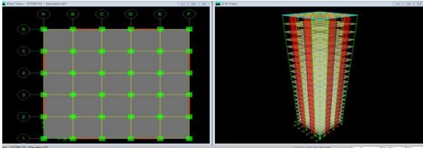
Fig.3 Shear wall at alternative positions
