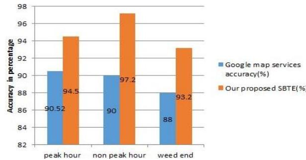
Fig. 4.4: Comparison between Google Map Services Accuracy and Our Proposed Software-Based Traffic Estimation Accuracy (SBTE) in Various Time Periods.
