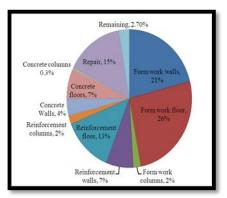
**Fig. 3:** Approximate relative breakdown of man-hours for a concrete structure (Lofgren and Gylltoft, 2001)
