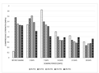
Figure 8: Compressive strength of CPC/PEG with the P/L ratio of 1.7 after soaking in Ringer's solution for 28 days.
