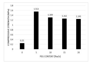
**Figure 6:** Effect of PEG addition on the compressive strength of CPC prepared with the P/L ratio of 1.7.
