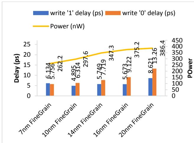
**Fig. 7:** Comparisons of Delay Time and Average Power Dissipation for Fine Grain Power Gating.
