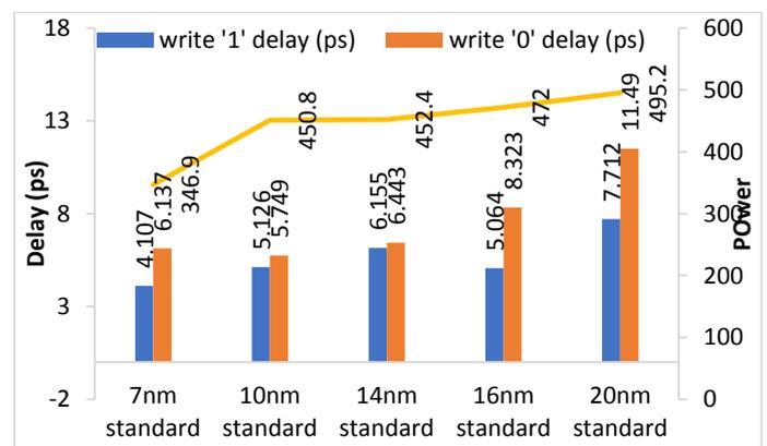
Fig. 6: Comparison of Delay and Power for Different Technology Nodes.
