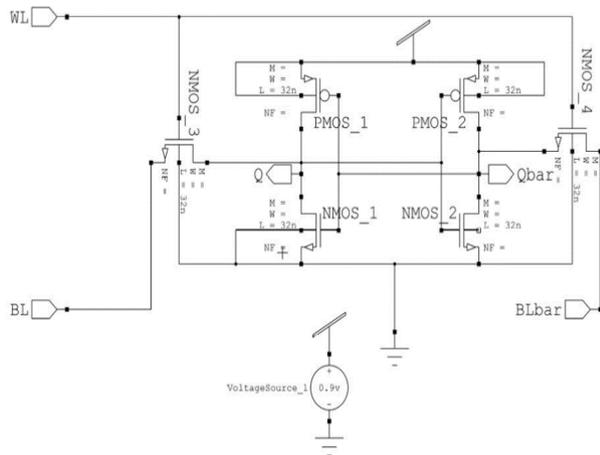
Fig. 4: The layout of FinFET based standard 6T SRAM cell in S-edit.
