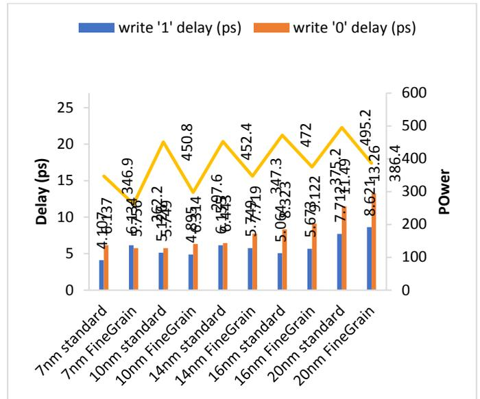
**Fig. 8:** Comparison between Standard Cell and Gated SRAM Cell for Each Technology Node.
