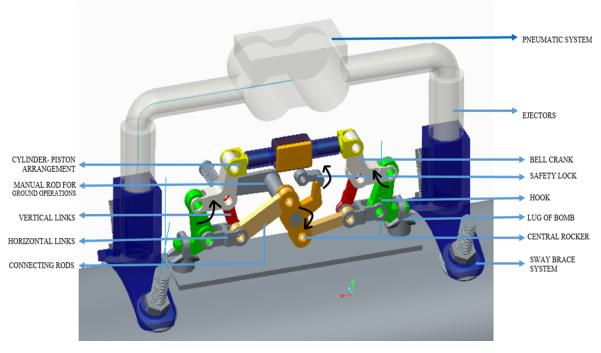
Figure 5: Developed Bomb Release Mechanism with sway braces and ejector unit
