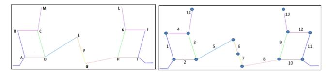
Figure 3: 2D geometry showing Links and Joints of BRM
