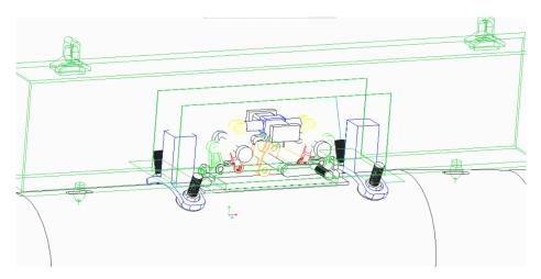
Figure 4: Geometric view showing pins of supporting frame which was inserted into the Bomb
