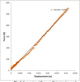
Fig. 4: Suspension stiffness coefficient testing result
