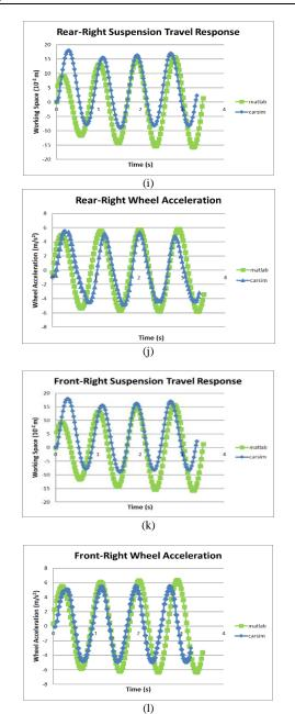
**Fig 5**: Validation graphic of: (a) body displacement response, (b) body acceleration response, (c) pitch angle response, (d) roll angle response, (e) front-left suspension travel response, (f) front-left wheel acceleration response, (g) rear-left suspension travel response, (h) rear-left wheel acceleration response, (i) rear-right suspension travel response, (j) rear-right wheel acceleration response, (k) front-right suspension travel response.
