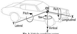
Fig. 1: Vehicle coordinate system
