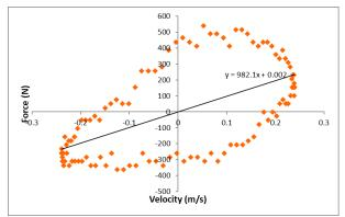
Fig. 3: Suspension damping coefficient testing result
