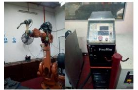
Fig 1: ABB IRB 2400/16 Robotic welding Machine (left) and KEMMPI ProMig 540 MXE (right)
