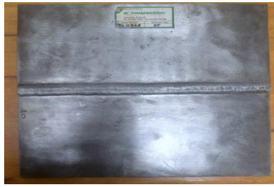
Fig. 3: Sample of Welded Flawed Specimen.
