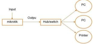
Fig. 1: Block Diagram of Large Scale Network (Wired).
