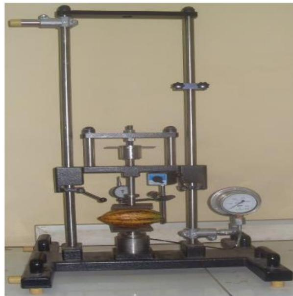
**Fig. 3:** Experimental Device Universal Testing GUNT HAMBURG (Model 198079) Used for Compressibility [15].
