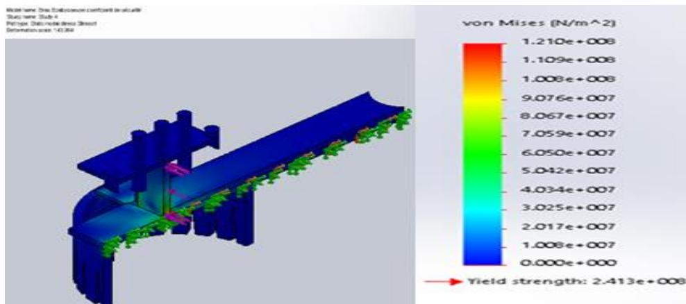
Fig. 7: Representation of the Stress on the Breaking Arm of the Cocoa Pod.
