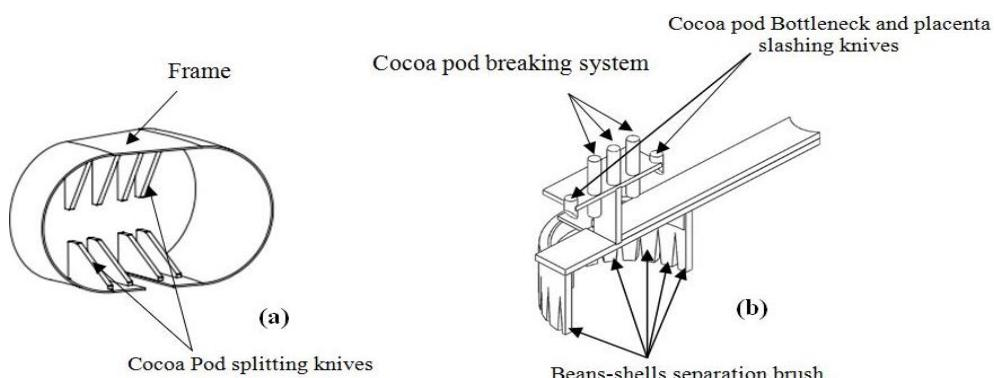
**Fig. 5:** Design of the Cocoa Pod Splitting Knives: (A) Cocoa Pod Splitting Frame and Knives (with Dimensions), (B) Cocoa Pod Slashing Knives Ready to the End of the Cocoa Pod.
