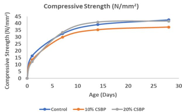
Fig. 3: The Compressive Strength Development of Concrete with CSBP Content.
