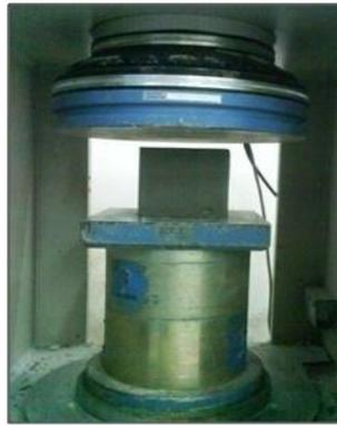
Fig. 2: Compressive Strength Test of Concrete Specimens
