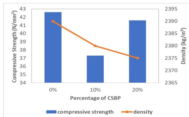
Fig. 4: The Compressive Strength of CSBP Concrete with Density at 28 Days.
