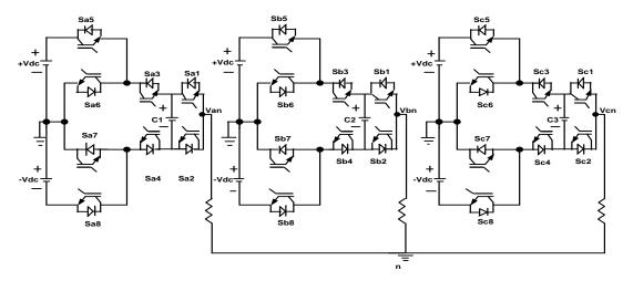
Fig. 17: Modified Circuit Diagram of Five-Level ANPC.
