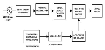
Fig. 27: Block Diagram of the Dc Power Supply Stage.
