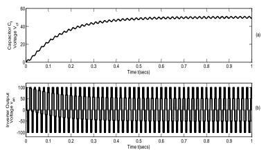
Fig. 18: (A) Capacitor voltage  $V_{cf}$  (B) Output load voltage  $V_{an}$  under self-capacitor voltage balance for the Type B hybrid multi-level inverter of Figure 17 with per cycle switch state sequence of  $1 \rightarrow 2 \rightarrow 4 \parallel 5 \rightarrow 6 \rightarrow 8 \& C_f = 7500 \ \mu F$ ,  $V_{dc} = 200 \ V$ ,  $F_C = 1.05 \ kHz$ ,  $F = 50 \ Hz$ , M = 0.8,  $Z_L = (5+20j) \ \Omega$ .
