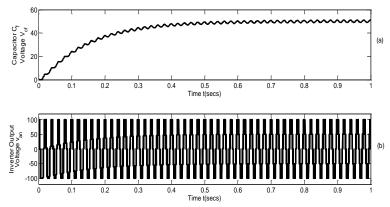
Fig. 19: (A) Capacitor voltage  $V_{cf}$  (B) Output load voltage  $V_{an}$  under self-capacitor voltage balance for the Type B hybrid multi-level inverter of Figure 17 with per cycle switch state sequence of  $1 \rightarrow 3 \rightarrow 4 \parallel 5 \rightarrow 7 \rightarrow 8$  & C<sub>f</sub> = 7500 µF,  $V_{dc}$  = 200 V,  $F_C$  =1.05 kHz, F = 50 Hz, M = 0.8,  $Z_L$  = (5+20j)  $\Omega$ .
