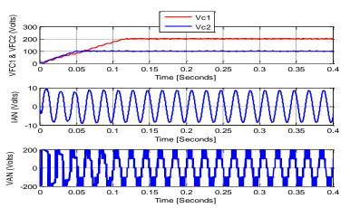
Fig. 5: (A) Capacitor voltages  $V_{c1}$  and  $V_{c2}$ . (B) Inverter output current ( $I_{an}$ ); (C) Inverter output Voltage ( $V_{an}$ ) under a balanced capacitor voltage control for Type A hybrid five-level inverter  $V_{dc}$  = 400 V,  $F_C$  = 5 kHz,  $F_s$  = 50 Hz, M = 0.8, with zero pre-charged capacitor voltage.
