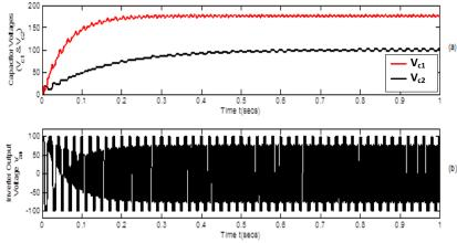
Fig. 3: (A) Capacitor Voltages  $V_{c1}$  and  $V_{c2}$ . (B) Inverter Output Voltage ( $V_{an}$ ) for An Unbalanced Condition of Type A Hybrid Five-Level Inverter  $V_{dc} = 200 \text{ V}$ ,  $F_C = 5 \text{ kHz}$ ,  $F_s = 50 \text{ Hz}$ , M = 0.8.
