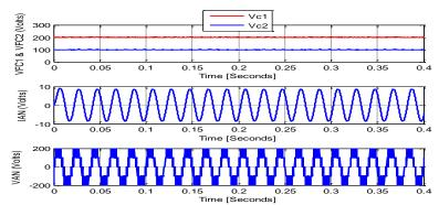
Fig. 6: (A) Capacitor Voltages  $V_{c1}$  and  $V_{c2}$ . (B) Inverter Output Current (I<sub>an</sub>). (C) Inverter Output Voltage (V<sub>an</sub>) Under A Balanced Capacitor Voltage Control For Type A Hybrid Five-Level Inverter  $V_{dc}$  = 400 V,  $F_C$  = 5 kHz,  $F_s$  = 50 Hz, M = 0.8, with 100 V And 200 V Pre-Charged Capacitor Voltage.
