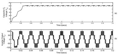
**Fig. 20:** (A) Capacitor Voltage  $V_{Cf}$  (B) Output Load Voltage  $V_{an}$  Under Natural Capacitor Voltage Balance for the Type B Hybrid Multi-Level Inverter of Figure 17 with Per Cycle Switch State Sequence Of  $1 \rightarrow 2 \rightarrow 3 \rightarrow 4 \rightarrow 5 \rightarrow 6 \rightarrow 7 \rightarrow 8$  And  $C_f = 1500 \mu f$ ,  $V_{dc} = 200$  V,  $F_C = 1.05$  Khz, F = 50Hz, M = 0.8,  $Z_L = (8+6j) \Omega$ .
