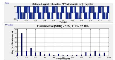
Fig. 25: Phase Voltage  $V_{an}$  of five-level ANPC inverter of Figure 17 with A Shorted Capacitor  $V_{dc} = 400V$ ,  $F_C = 5$  kHz, F = 50Hz, M = 0.8,  $Z_L = (8+6j) \Omega$ .
