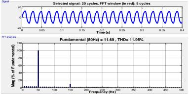
Fig, 13: Three Level Phase Current (Ian) With A Bypassed H-Bridge And Full Power.
