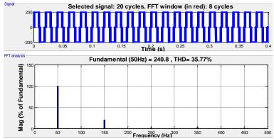
Fig. 14: Three Level Phase Voltage (Van) With A Bypassed H-Bridge And Full Power.
