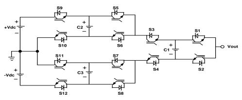
Fig. 16: Circuit Diagram of Five-Level ANPC.
