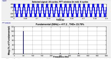
Fig. 15: Three Level Line-Line Voltage (VAB) With A Bypassed H-Bridge And Full Power.
