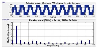
Fig. 26: Lines AB Voltage  $V_{AB}$  of five-level ANPC inverter of Figure 17 with A Shorted Capacitor.  $V_{dc} = 400V$ ,  $F_C = 5$  kHz, F = 50Hz, M = 0.8,  $Z_L = (8+6j) \Omega$ .
