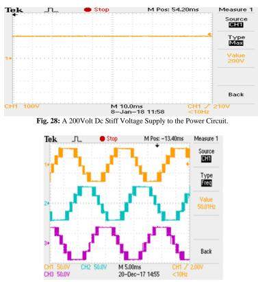
Fig. 29: Five Level Phase Voltage at 1.2 MI.
