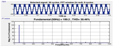
Fig. 7: Phase A Output Voltage ( $V_{an}$ ) with A Balanced Capacitor Voltage for Type A Hybrid Multi-Level Inverter of Figure 1.  $V_{dc}$  = 400 V,  $F_C$  = 5 kHz,  $F_s$  = 50 Hz, M = 0.8,  $Z_L$  = (8+6j)  $\Omega$ .
