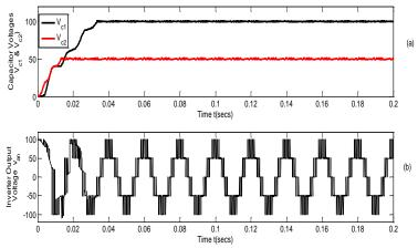
Fig. 4: (A) Capacitor Voltages  $V_{c1}$  and  $V_{c2}$ . (B) Inverter Output Voltage ( $V_{an}$ ) for a balanced Condition of Type A hybrid five-level inverter,  $F_C = 5 \text{ kHz}$ ,  $F_s = 50 \text{ Hz}$ , M = 0.8.
