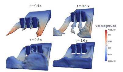
Fig. 3: Simulation results for cylinder obstacle at t = 0.4 s, t = 0.6 s, t = 0.8 s, and t = 1.0 s.
