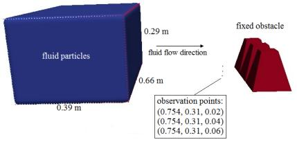
Fig. 1: Initial setup of dam break simulation with 128309 SPH fluid particles.
