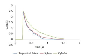
Fig. 6: Velocity in x axis direction (vx) at point (0.754, 0.31, 0.02) for the various obstacles.
