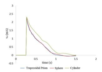
Fig. 8: Velocity in x axis direction (vx) at point (0.754, 0.31, 0.06) for the various breakwaters.
