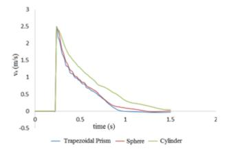
Fig. 7: Velocity in x axis direction (vx) at point (0.754, 0.31, 0.04) for the various obstacles.
