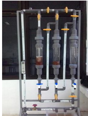
Fig.1: Fixed-Bed Column used to experiment
