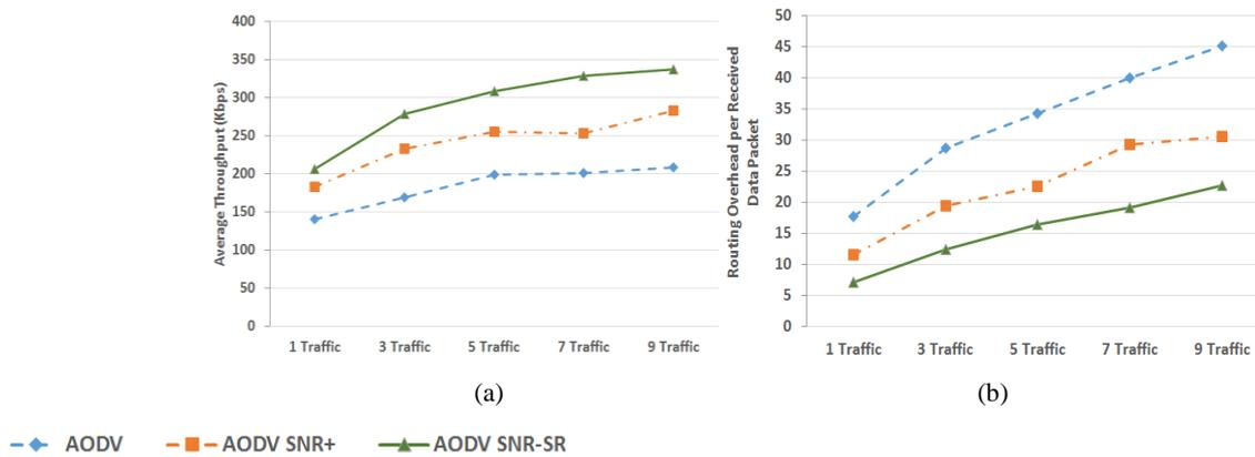
**Figure 4:** Average throughput (a) and routing overhead (b) comparison between AODV, AODV SNR-SR, and AODV SNR+ with increasing number of traffic source
