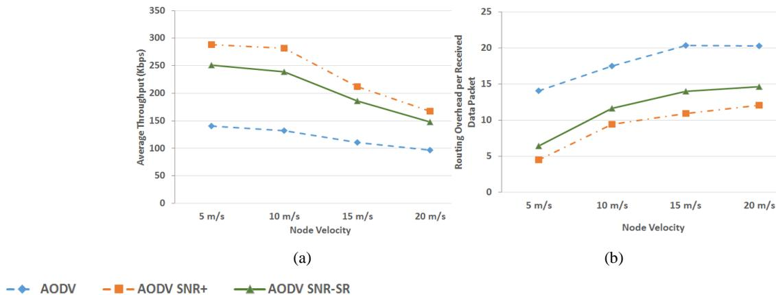
**Figure 5:** Average throughput (a) and routing overhead (b) comparison between AODV, AODV SNR-SR, and AODV SNR+ with increasing node velocity.
