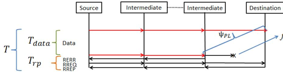
Fig. 1: The model of routing protocol AODV with path life.
