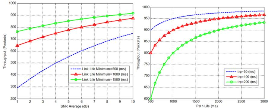
Figure 2: Throughput performance (a) with SNR average and the link life minimum (b) with path life and time to repair broken path.
