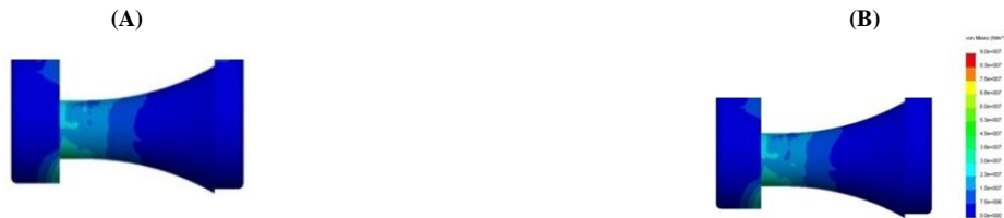
Fig. 13: Von Mises Stress Plot for Modified Humeral Component Related to Different Polyethylene Bushing Sizes in Case 3 (A) Case 3A (B) Case 3B.
