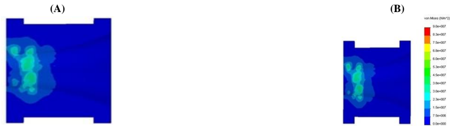
Fig. 10: Von Mises Stress Plot for Different Polyethylene Bushing in Case 3 (A) Case 3A (B) Case 3B.
