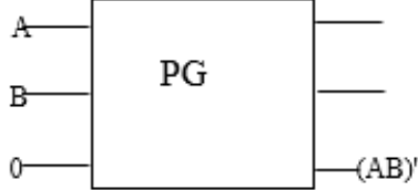
Fig. 2: Peres Gate as NAND Gate.
