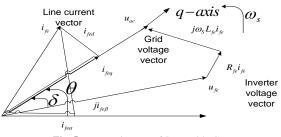
Fig. 5 Vector Diagram of Stator side Converter cross-coupling terms ( $\omega_s Lf_e i_{fed}$  and  $\omega_s L_{fe} i_{feq}$ ) and disturbance input
