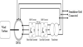
Fig. 1 DFIG connected Wind Turbine
