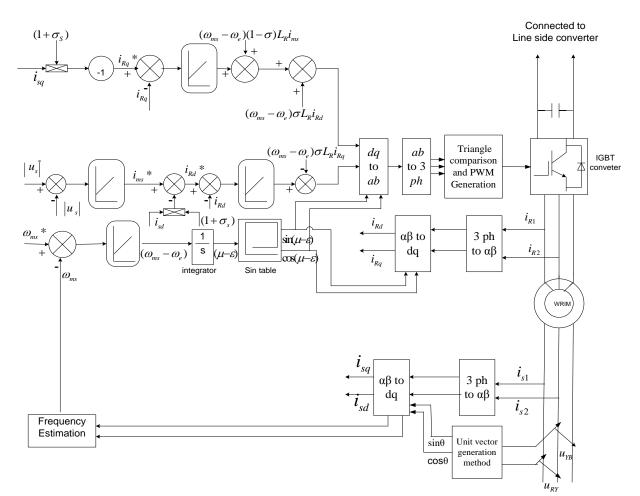
Fig. 4 Block Diagram of Rotor side Converter
