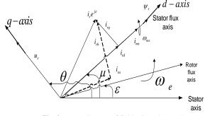
Fig. 2 Vector diagram of field oriented control
