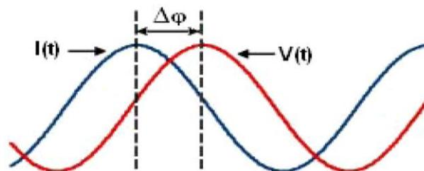
Fig. 3: Phase shift between Current  $I(t)$  and Voltages  $V(t)$  in AC Line before Rectifier.
