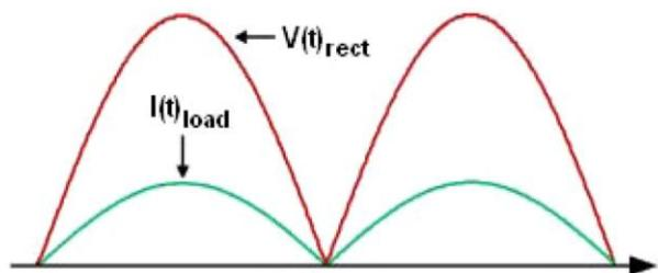
Fig. 4: Phase of Current  $I(t)_{load}$  and Voltage  $V(t)_{rect}$ .
