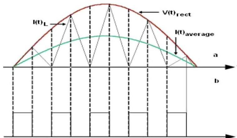
Fig. 6: Timing Diagram of PWM signal 'b' for Driving MOSFET Transistor Accordingly to Amplitude of Rectified Voltage  $V(t)_{rect}$  and Current Across Choke Coil  $I(t)_L$  'a'.
