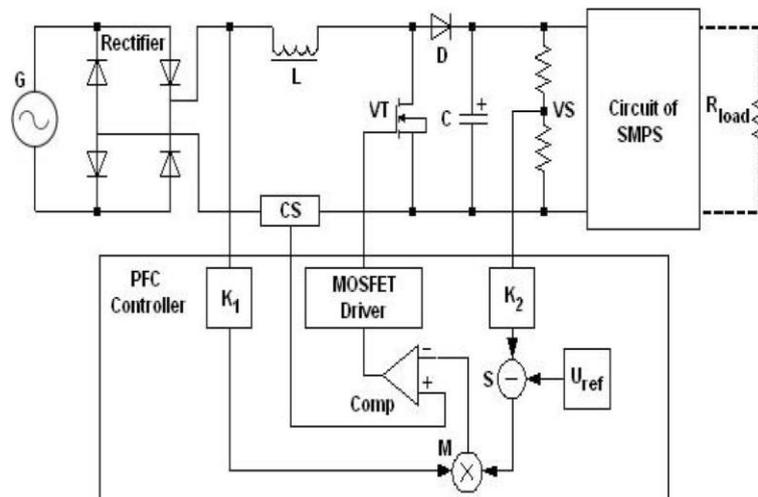
Fig. 5: Simplified Electronic Power Circuit of the Active PFC.
