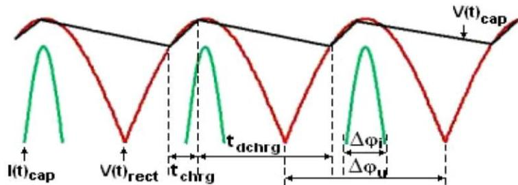
Fig. 2: Waveshape of fully Rectified Voltage  $V(t)_{rect}$ , Current  $I(t)_{cap}$  and Voltage  $V(t)_{cap}$  across input Capacitor (C).
