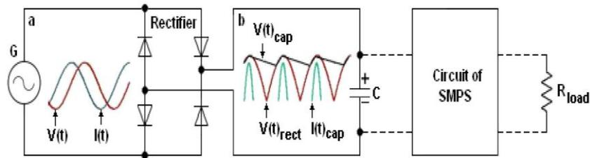
Fig. 1: Input Circuit of the SMPS.
