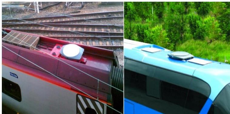
Fig. 10: The Phased Antenna Array Installed on the Roof of the Train and Bus.
