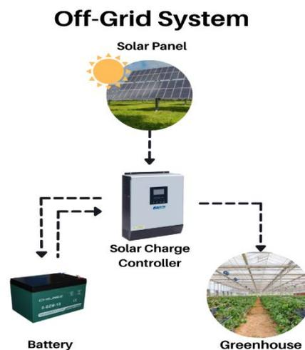
Fig. 2: Off Grid System Where Inverted Was Functioned as Solar Charge Controller.
